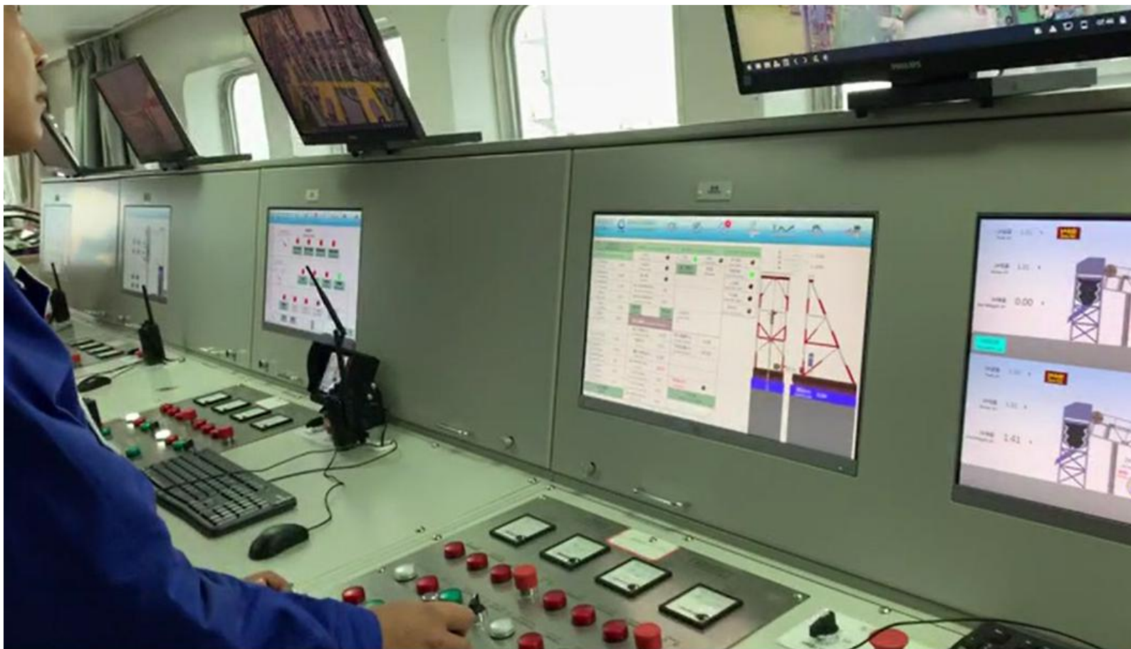
Center Control Room in Cabin Realize Automatic Pile Making
